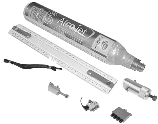
Fig. 9. Pneumatic components and a 30 cm ruler to indicate their sizes. The components are clockwise arranged according to the CO 2 flow through the system; 5.8 MPa CO 2 canister, the first-stage pressure regulator to 1.2 MPa, a block of four second-stage regulators to 0.6 MPa, one of four low-power SMC valves, one of four small SMC cylinders, and one of four Shadow McKibben muscles.
